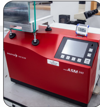
Fine leak testing
