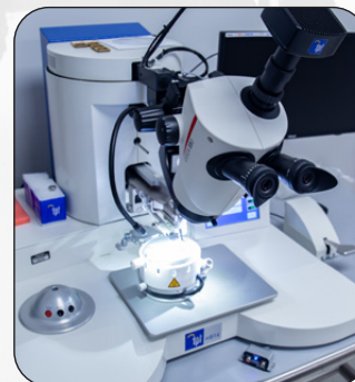
Semi-automatic die attach and wire bonding
